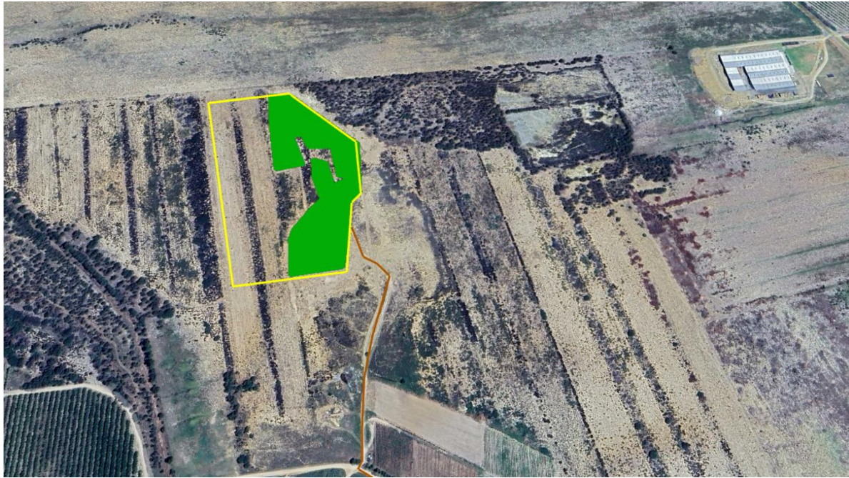
Figure 1: Image taken from the Google Earth 2026 showing the mining area with the disturbed and rehabilitated area. The approved mining area was 4.9 ha in extent with approximately 2 hectares thereof disturbed. The Rehabilitation, Decommissioning and Mine Closure Plan details the closure objectives, -actions, relinquishment criteria, monitoring, auditing and reporting commitments for the earmarked area. The green polygon was added to indicate the affected and rehabilitated areas.
